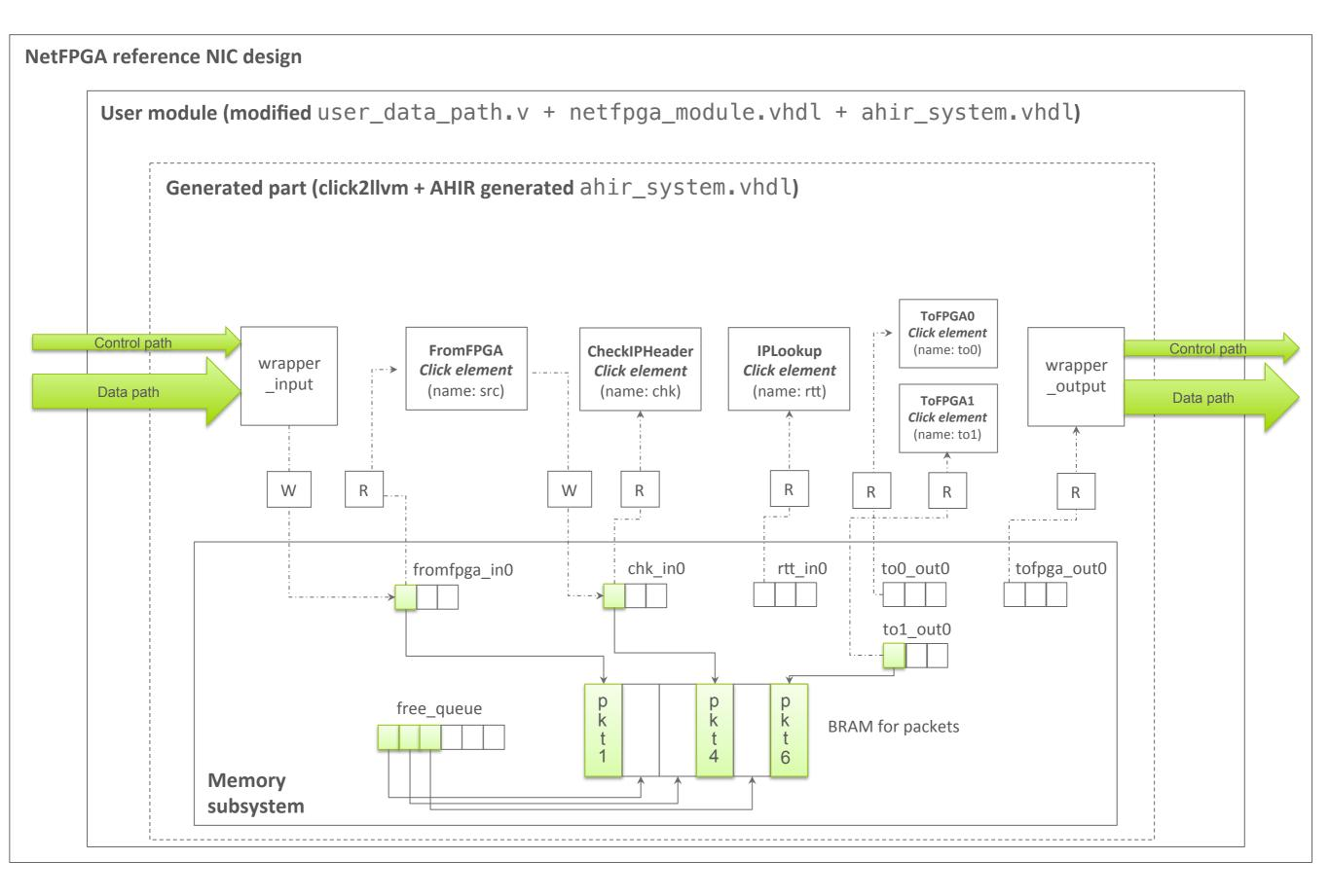
NOTE: Click elements are running in parallel, each processing a different packet, while software Click operates in run-to-completion mode.
