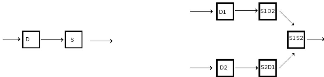
Figure 2: The different states of a single peer in a single-chunk and two-chunk Markov chain model. D represents the download of a chunk while S represents seeding. In the single-chunk model, peers will always enter the system as downloaders, then become seeds before leaving the system. In the two-chunk model, peers can start downloading either of the two chunks, before becoming an uploader for the downloaded chunk and a downloader for the other chunk. They then become seeders who share both of the chunks before departing the system.
